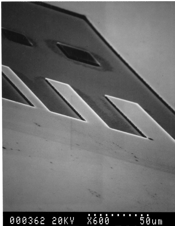
Figure 5 SEM micrograph of cantilever microbeams.
